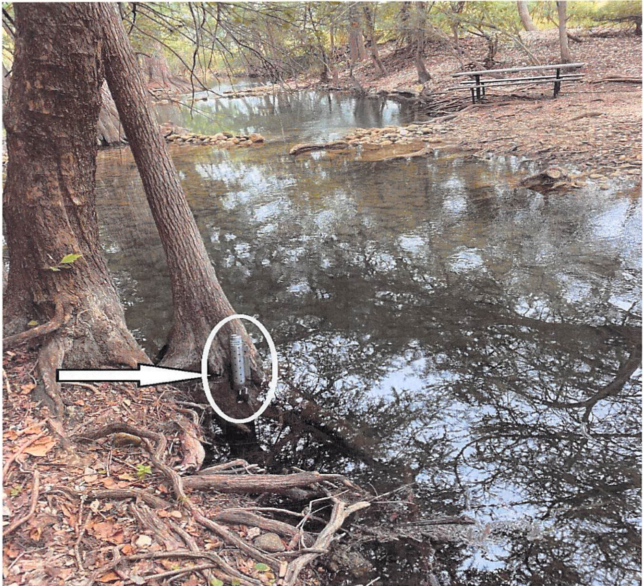
Figure 2: One of Five USGS In-situ Pressure Transducer, Water Level Electronic Data Loggers installed above Utopia, Tx. along the Sabinal and West Sabinal Rivers.
